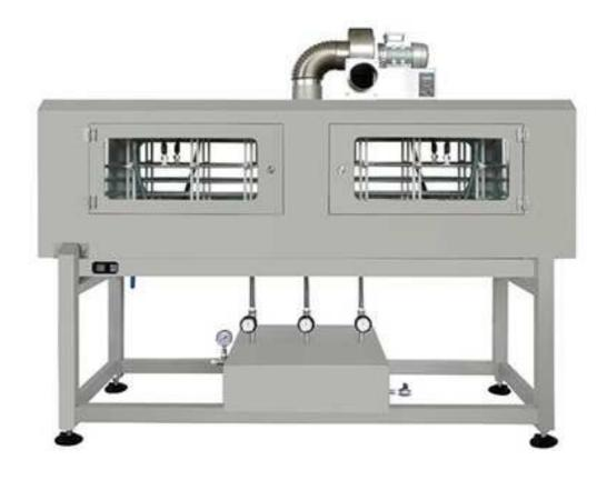
Steam shrink tunnel is used for shrinking sleeve labels to label kinds of bottles: different and irregular round bottles, square bottles, flat bottles and women-shaped bottles. By shrinking PVC or PET sleeve labels to seal bottles caps /necks, cover bottles body even shrink wrap bottle bottom.
