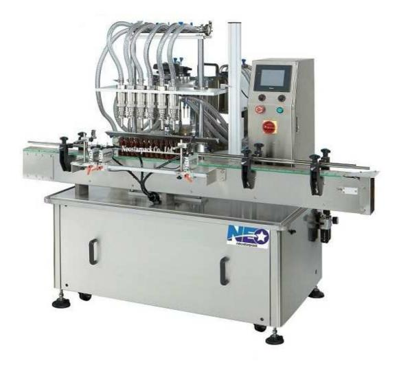
Automatic 6-Nozzle Overflow Liquid Filler NFL-465 is best suitable for filling with foamy, flammable, corrosive liquid products, or products which require consistent filling level. The number of nozzles can be customized according to your needs, and the filler can also be connected with other packaging machines to build up a complete production line.
