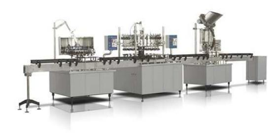
This filling machine include ZC auto washer, GD balanced pressure filer, WFG cap turning machine, SSJ carrying machine etc. The key parts are made of stainless steel, with the features of reasonable structure, advanced technology, easy in operation, widely used, etc, it's the ideal production line for middle and small drink factory.
