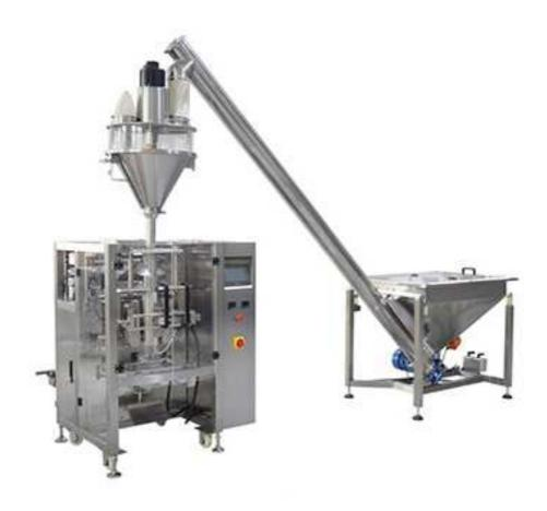
VFFS Vertical Full Automatic powder packaging machine is suitable for packing fine dry powder materials, such as milk powder, spices powder, coffee powder, corn flour, laundry powder, coconut powder, fruit powder, collagen protein powder, cocoa powder, chili powder, etc.
