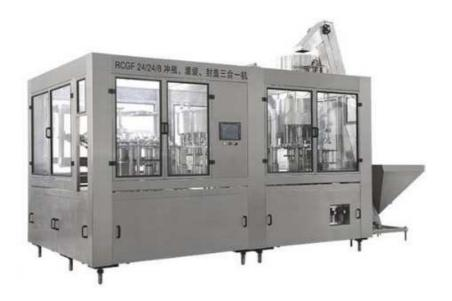
3-in-1 filling machine, combined with rinsing, filling and capping. It is innovated and designed in the requirement of still pure water and mineral water, on the bases of introducing, digesting and absorbing advanced technology from Germany and Italy.
