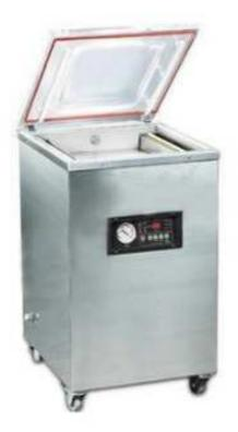
The packaged products can be prevented from oxidation, going mould, insects or getting damp, thus can be kept fresh after closing the lid, the machine can automatically run through the full cycle of installed functions, including vacuum extraction, insert gas flushing (optional), sealing, printing, cooling and exhaust. The packaged products can be prevented from oxidation, going mould, insects or getting damp, thus can be kept fresh in a prolonged storage time.
