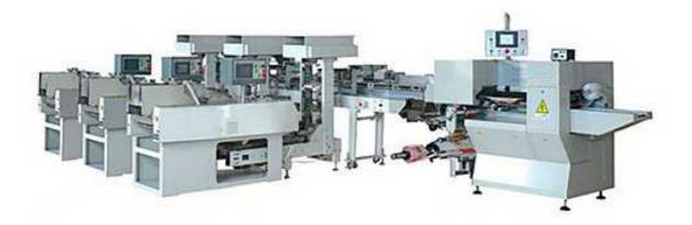
Our noodle packing machine can automatically finish the process of weighting, outputting, filling and sealed packing of noodles and spaghetti
