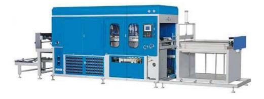
JH711/1200-A Automatic Vacuum forming machine with big forming area is designed by the principle of mechanical-electrical-pneumatic integration. It adopts PLC control system, panel and digital power control. This full-automatic forming equipment for forming plastic sheet includes feeding, heating, forming, cooling, mold ejecting, cutting at one blow. This machine has luxury configuration and gets reliable performance and handy operation.
