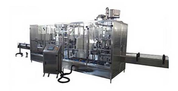
3L-10L water filling machine can be classified into atmospheric pressure filling machine and isobaric pressure filling machine. It depends on the production that customers want to produce. Generally mineral water production line, and pure water production line will choose atmospheric pressure filling machine. Carbonated drink production line, oil production line and fruit juice, fruit tea production line will choose isobaric pressure filling machine.
