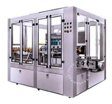
This is a helicoids bottles rinse machine, it adopts continual tracking to spray and wash bottles, high efficiency, well effect of rinse, it is suitable for different specifications of bottles. Widely range, easy operating convenient maintaining.
