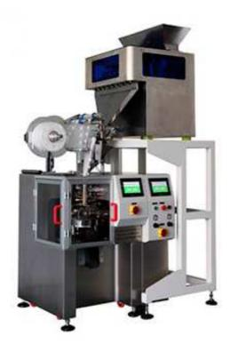
KST-LX12, The latest design high speed pyramid tea bag packing machine, adopts the unique Resonance Sealing Structure, the Max working speed reaches 120 bags/min. Equips with the high accurate linear weighed & two times feeding system, it was specially design for the enterprises with large output.
