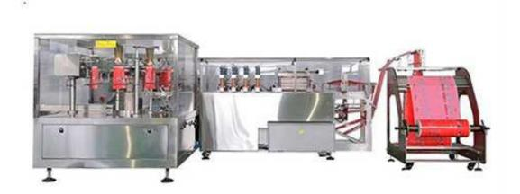
Pre-made pouch rotary machine suitable for powder, particle, solid, liquid, thick, tablet packaging
