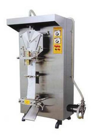
The machine is widely used in water, milk, soy milk, all kinds of beverages, soy sauce, vinegar, rice wine and other liquid film packaging; UV sterilization, bag in full bloom, print date, quantitative filling, sealing cut off, automatic counting one-time automatic Complete, heat sealing temperature using automatic control, packaging products beautiful and reliable, shell, pipe, sterilizer, quantitative pump with stainless steel structure to ensure health.
