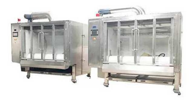
LST Belt Chocolate Coating machine and Chocolate Polishing machine are mainly used for making chocolate bean products stuffed with peanuts, almonds, raisin, puffed rice balls, jelly candies, hard candies, QQ candies etc. LST made the first Belt Chocolate Coating Machine in China. We have been constantly improving it over the past few years. It is durable and works perfectly.
