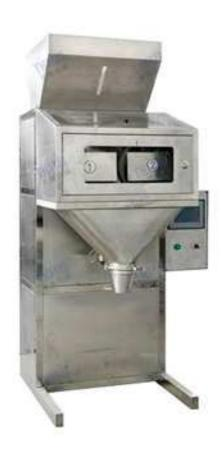
The rice bagging machine can complete automatic bottle positioning, filling and metering. It is controlled by PLC and touch screen, which is easy to operate and has high stability. The touch screen can be customized for different language. The machine doesn't has any requirement about the bag, you can choose any type bag.
