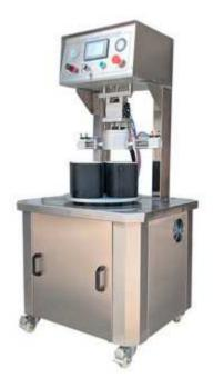
Vacuum capping machine generally refers to the equipment used for glass bottle tinplate capping vacuum packaging equipment. The glass bottle mouth is spiral, the cap is usually made of tinplate, with the same number of buckles as the corresponding bottle mouth thread, according to different bottle mouth diameter standards for three, four, six buckles of the cap, respectively matching the corresponding number of spiral glass bottles.
