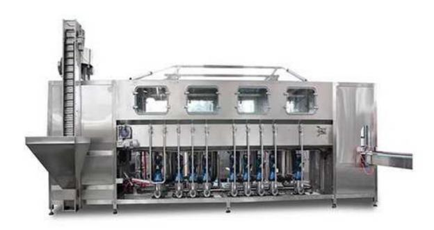
QGF Series barrel machine is specially used for 3/5 Gallon barrel drinking water. This machine combined washing/filling/capping into one machine. Mainly used for filling mineral water/distilled water/pure water and so on.
