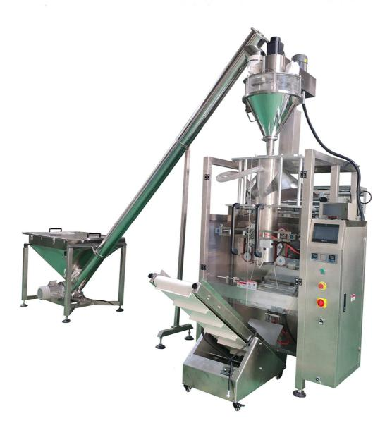
The 5kg powder packaging machine is used for one of a big flour powder factory package solution of almost all the packaging is 5kg pillow bag for baked flour, then some package packed into a carton for safe and sanitary transport. Sure, the machine can pack smaller package, such as 3KG, 4KG etc by changing different bag former if the bag width is different, and the bag length is always adjustable on the HMI touch screen.
