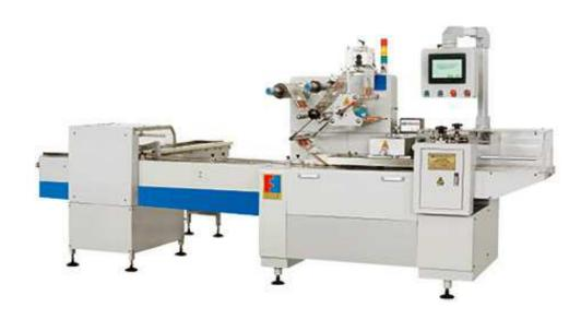
FFW is the equipment for biscuit on edge packing machine without tray, it saves the huge manpower and material cost for our clients suitable for fast packaging of the biscuit, wafer and other slice, round and regular items without tray.
