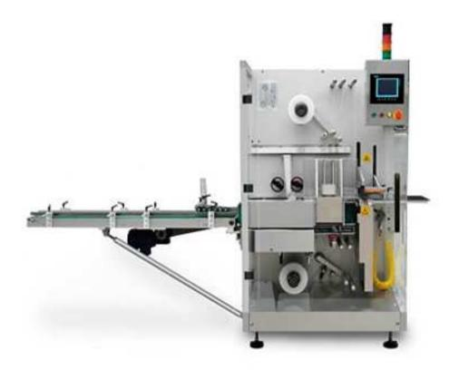
Auto high speed Bundling machine BC240, up to 40 bundles/min
