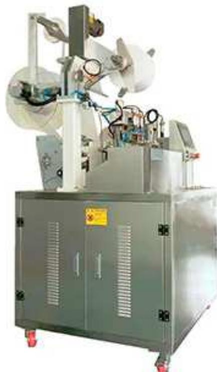
This is our labeling and tagging machine, the machine adopt ultrasound sealing, it makes nylon tagged mesh with thread and tag, and making roll tagged material used on the pyramid tea bag packing machine. It is suitable for different material like Nylon mesh, biodegradable PLA corn fabric mesh, non woven mesh, PET mesh etc.
