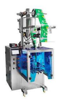
Liquid Irregular Bag Packing Machine is suitable for metering and packaging of liquid and sauce in food, pharmaceutical, chemical and cosmetic industries. The packaging material can be PE composite film, such as pure aluminum, aluminized, nylon, etc. All the work of bag making, measuring, filling, sealing, cutting and counting can be done automatically, meanwhile, it can also be customized to print batch number and other functions.
