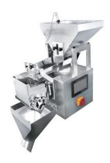
The single head linear weigher is designed for the weighing of tiny granules with a diameter lower than 20mm such as seeds, white sugar, dried fruit, washing powders and more. This linear weigher features an easy product and target weight change, making it suitable for packaging in different target weights and several uniform granules. The remote control via internet is easy and efficient to use.
