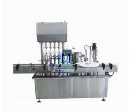
The Paste Filling and Capping Machine (high viscosity, low fluidity) has an improved common filler, mainly for high viscosity, low fluidity products. Different speed grades are available for customized requirements. It can be used as a standalone or connected to other machines as an integral production line.
