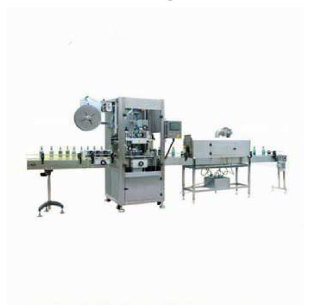
Synchronized transmission, any change of transmission belt will be finished quickly. Compared to the type of traditional multilayer whose change and maintain need more than six hours, it's maintenance is easy and maintain is simple, so it doesn't influence production.
