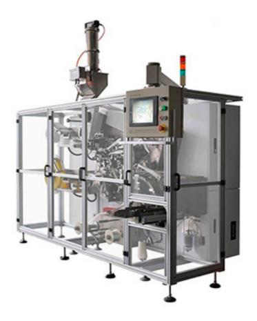
The machine DXDC10 is a kind of automatic tea bag machine for the packing of tea and similar Chinese herbs / Flower tea. It makes double chamber tea bags which are cold-sealed. The machine links up hard label and thread with staple, and the tea bags are pushed out and packed into box manually after counting. The packing materials are non-heat-sealed filter paper, label, thread and staple.
