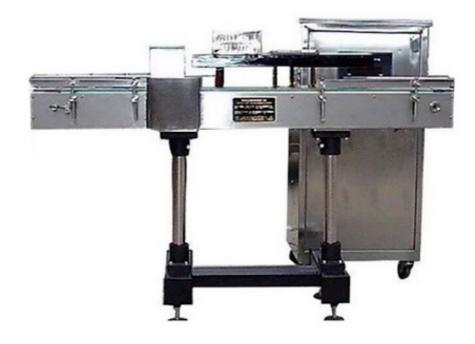
It is new generation production which adopts electromagnetic induction technical. The machine is economical and easy to operate. It uses widely in food& beverage, Pharmaceuticals and chemical industry etc. This fully automatic sealing machine can seal the mouth of container with aluminum foil at speeds up to 60 cpm.
