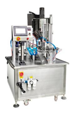
This machine is the mufti-functional and advanced yogurt cup filling machine. It is featured with automatic dispensing glass, filling, sealing, cover pressing. It is suitable to milk, juice, honey, water and granular, powder, fruit, crisp and so on.
