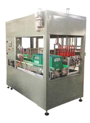
This is an intelligent fully automatic carton packing machine, controlled by PLC and friendly Human machine interface. With functions such as: Machine automatic stop if lack of bottles, no bottle no packing. Greatly reduce the labor force; it is a nice equipment to be working on the automatic line.
