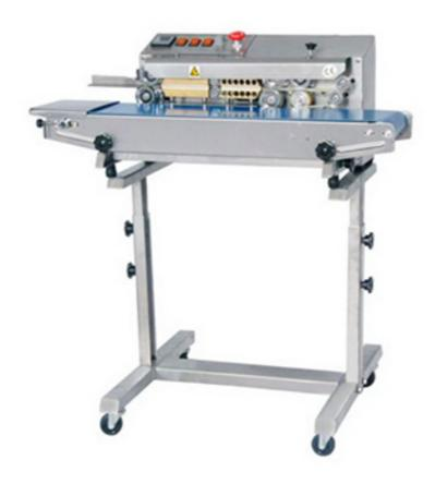
The machine is ideal for sealing small packages, which adopts constant temperature control system and stepless speed regulation mechanism.
