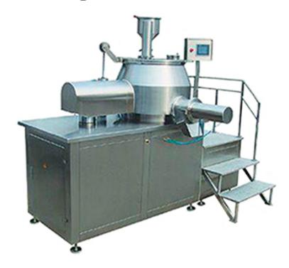
The powder raw material and adhesive in a cylinder are mixed fully at the bottom to become a humid soft material. The it is cut through high-speed crusher and become uniform granules.
