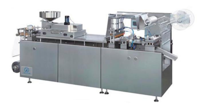
DPP-250DII Automatic Blister Packaging Machine is designed according to the GMP standard, and this machine is widely used for alu-alu Packaging capsules, tablets in the pharmaceutical industries.
