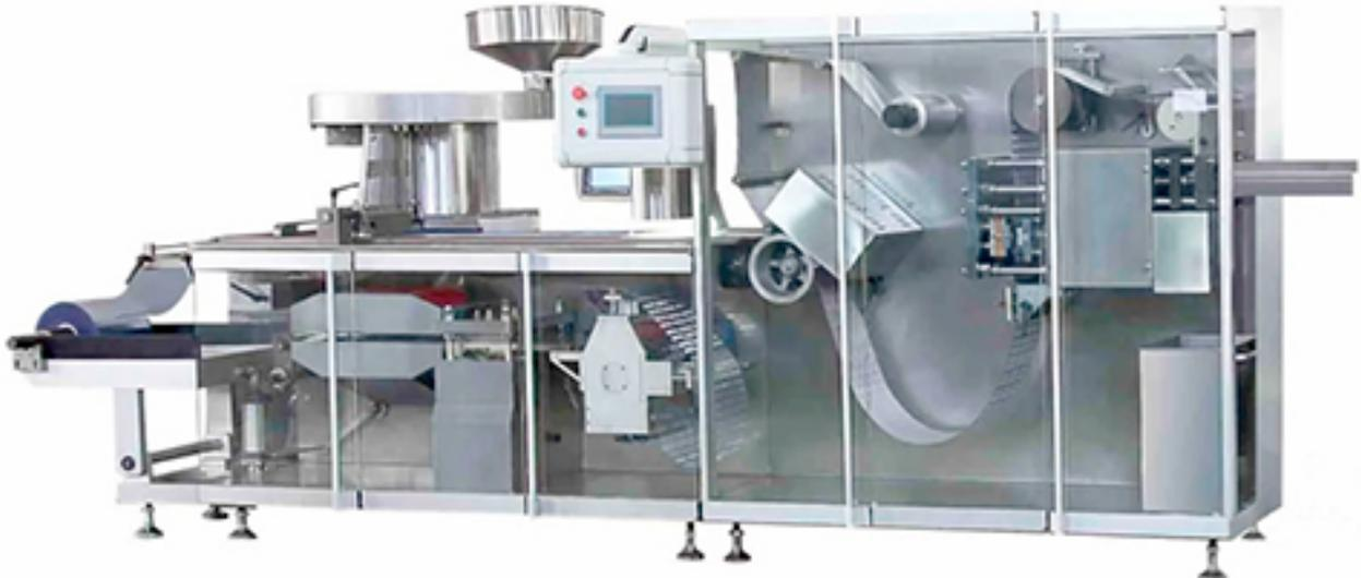
DPH260H highly intelligent high-speed roller blister packaging machine is used for blister-type aluminum (PTP)/plastic (PVC) composite sealing packaging of medicines (tablets, capsules), food, medical equipment, health products, electronic components and similar materials. Special equipment, due to the use of positive pressure forming and rolling heat sealing, it has the characteristics of crisp blister and flat plate.
