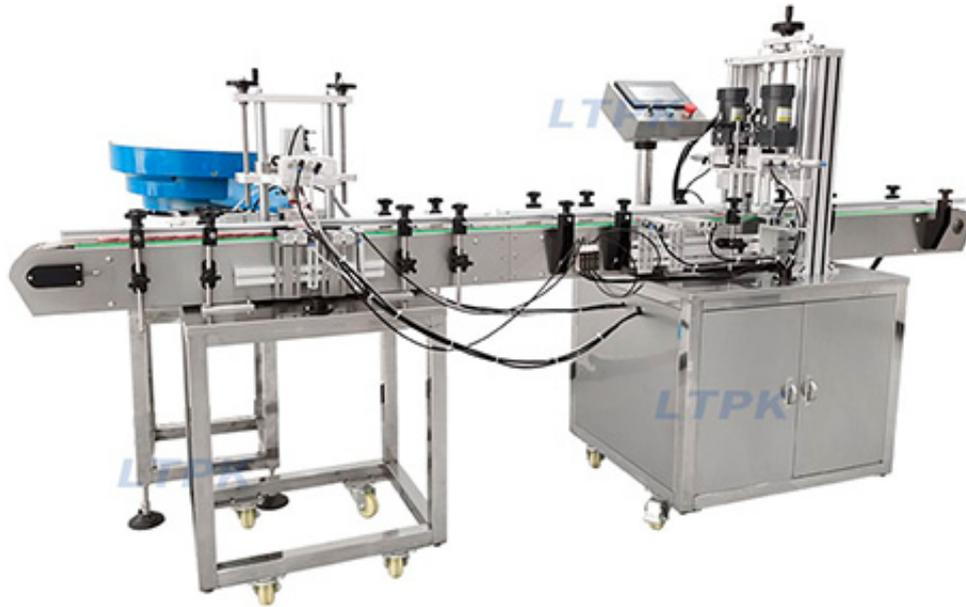
This full automatic capping machine is equipped with a cap feeder, which can orient bottle caps. Typically the cap feeder can be customized by making adjustments to the bowl for different sizes of caps. Larger caps and higher speeds may require larger bowls. These two machine can achieve automatically feeding caps and cap bottles, save labor and reduce production error.
