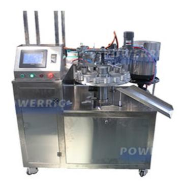
It can be used to fill and seal plastic bottles, mainly used for super glue, 502 glue, cyanoacrylate glue and other products. This machine has a working plate and two vibrating plastics (based on the cap), with filler heads and 16 positions.
