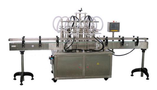
This machine is widely used filling liquid, semifluid liquid, such as liquid soap, shampoo, oil, and so on.
