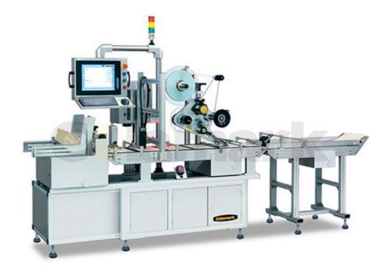
The A3 series personalizes and labels cards/sheets of size from CR80 to A4. Different printing technologies including CIJ, TIJ, DOD or laser printers can be seamlessly integrated. It also consists of labeling engine for scratch off label or other identification labels application, vision inspection and diversion devices for data integrity control. An ideal equipment for scratch cards, contact and contactless smart cards, forms and tickets etc.
