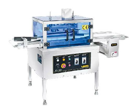
The RC-180 is designed to roll food products into a ball. After putting food products on the conveyor, the machine can convey food products to the working area for rolling. It can work with Automatic Encrusting and Forming Machine series (SD-97W/SD-97SS/SD-97L) to roll the quantitatively-divided filled or non-filled food into a ball.
