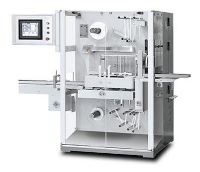
HB 40 is an automatic stretch banding and shrink wrapping machine for cartons. Its balcony design allows maximum accessibility to all main parts for optimizing maintenance and increases operator friendly environment through PLC control system with a touch panel.
