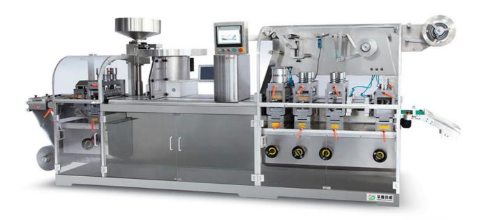
Forming mould, heat-sealing mould, batch number emboss printing mould and punching mould adopt drawer type mould change with national patent to achieve high efficiency.
