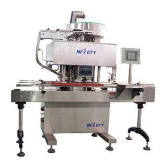
Exclusively used in threaded plastic caps automatically feeding, Sorting, caps dropping and capping process.
