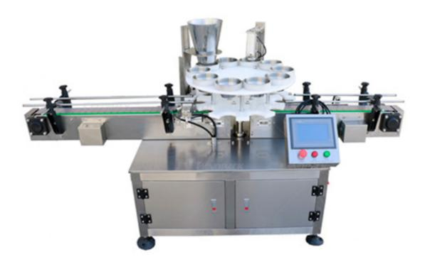
Suitable for filling granular products such as nuts, popcorn, potato chips, puffed food, peanuts, beans, capsules, tablets ect.
