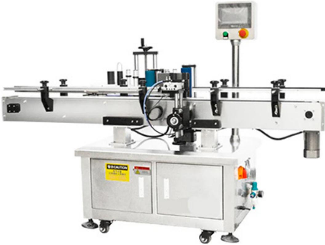
The automatic round bottle labeling machine is designed to apply labels accurately and efficiently on cylindrical or round-shaped containers. This machine is widely used in industries such as food and beverage, pharmaceuticals, cosmetics, and chemicals, where labeling accuracy, speed, and consistency are essential for round bottles or jars in large-scale production environments.
