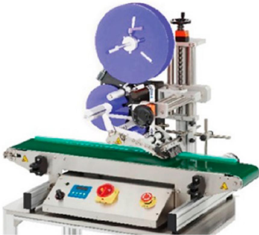
The ALT1100 is a compact, high-efficiency tabletop flat surface labeling machine, perfect for labeling foil bags, plastic bags, paper boxes, and meal boxes. Equipped with a high-precision imported photo-eye and stepper motor, it ensures fast and accurate labeling. The brush and sponge roller design guarantees smooth label application without lifting edges.
