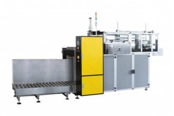
Case equipment is used to erect, pack, seal, or unpack cases of products. In most instances, case equipment is used to form cardboard boxes; however, corrugated materials and plastics formers are also available. Types of case equipment include case erectors, case cartoners, carton packers, carton sealers, and unpackers.
