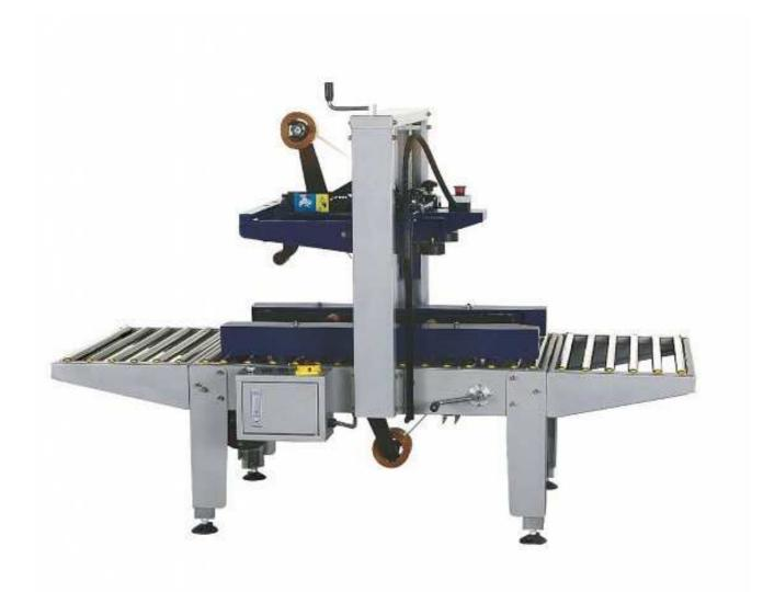
Carton sealers are case equipment that seals the top or bottom of a case with tape or glue. Typically, the minor corrugated flaps are kicked and plowed closed as the cases are transferred. As the cases enter the compression section, the major flaps of the carton are closed and a hotmelt adhesive is applied.
