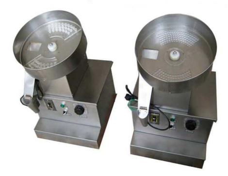
This machine applied to pharmaceutical, hospital, food etc industries, to the capsule, tablet, grain etc pharmacy or food counting. Whole machine made by stainless steel, the cubage is small, weight is light, counting is accurate, and operation is freely. Is the perfect machine to relate industry bottle packing, bag packing, can packing etc.
