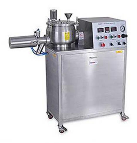
Pilot scale rapid mixer is mainly used in R&D or F&D facility for the wet mixing of the pilot batches. Basically, it consists of a Bowl, Impeller & Chopper assembly.
