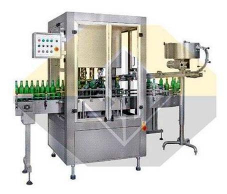
VCY-8 Automatic Chuck Capping Machine is special designed for cylinder bottles. It uses plastic inner cap and outer cap for capping. The max capping speed can reach 100 bottles/min.
