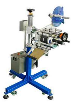
HL-T902 on line labeling applicator, Can be related to the production line, the flow of products, on the plane, curved labeling, implementing online marking, realize supporting to spurt the code conveyor belt, the flow through the object labeling
